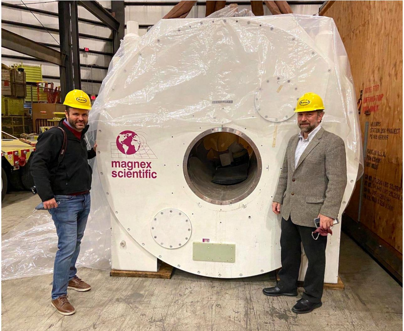
Fig. 1: 9.4T, 65cm bore magnet received at local warehouse. Alexandre Franco (L) and Thomas Vaughan (R) provide scale.
